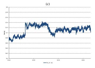
As soon as the voltage drops below 210V the charging power decreases from 3500W per phase to about 2600W. The current THD at this point rises from 4% to 6% while the THC stays constant at about 0.7A. Therefore, the reduction of the charging power does not decrease the harmonic load but leads to a lower power factor and lower efficiency.
