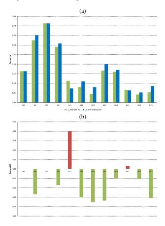
Figure 4 shows that the harmonic emissions of most odd harmonics are reduced if there is a PV system connected. Just a few odd harmonics are getting higher (H11, H21, H29, H47, H49). The reason for the change of the harmonic load is very likely the changed voltage harmonics due to the presence of the PV system.
