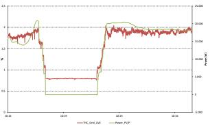
It can be seen that the harmonic load is reduced in the case the PV generation is zero. This leads to the statement, that the combination of a PV system and an EV charging station increases the amount of harmonic emission. The same behaviour can be seen in higher frequencies  $(2-9 \mathrm{kHz})$ .
