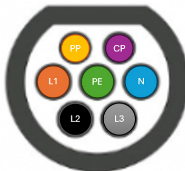
Fig. 1: SAE J1772 Type 1 connector pins
